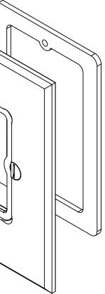
NOTES: 1.) COVER PLATE MATERIAL: BRASS, COVER PLATE MOUNTING SCREW MATERIAL: BRASS, GASKET MATERIALS: POLYURETHANE FOAM, O-RING MATERIAL: SILICONE 2.) WHEN USED WITH FB-5 FLOOR BOX IT IS UL LISTED, FLOOR BOX MEETS UL514C SCRUB WATER EXCLUSION TEST **EXCLUSION TEST**
