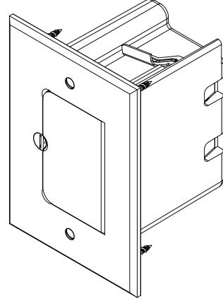
1.) BOX MATERIAL: POLYCARBONATE, COVER PLATE MATERIAL: DARK BRONZE PLATED BRASS, COVER PLATE MOUNTING SCREW MATERIALS: DARK BRONZE PLATED BRASS, DEVICE MOUNTING SCREW MATERIALS: ZINC PLATED STEEL, FLANGE MOUNTING SCREW MATERIALS: BLACK PHOSPHATE COATED STEEL WING
