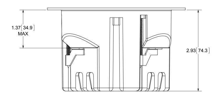
NOTES: 1.) BOX MATERIAL: POLYCARBONATE, WING MATERIAL: GALVANIZED STEEL, WING SCREW MATERIAL: ZINC PLATED STEEL 2.) UL LISTED WITH 2 HOUR FIRE RATING FOR WALL
