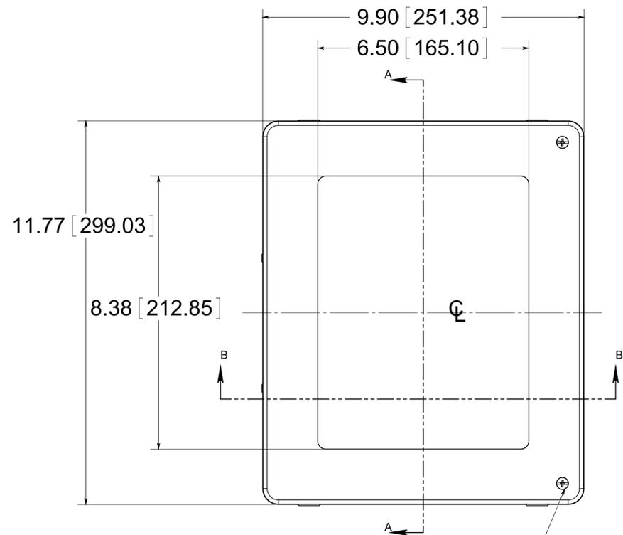
(2) EACH #10-32 BRASS INSERTS AND STAINLESS STEEL CAPTIVE COVER SCREWS WITH RETAINING O-RING
