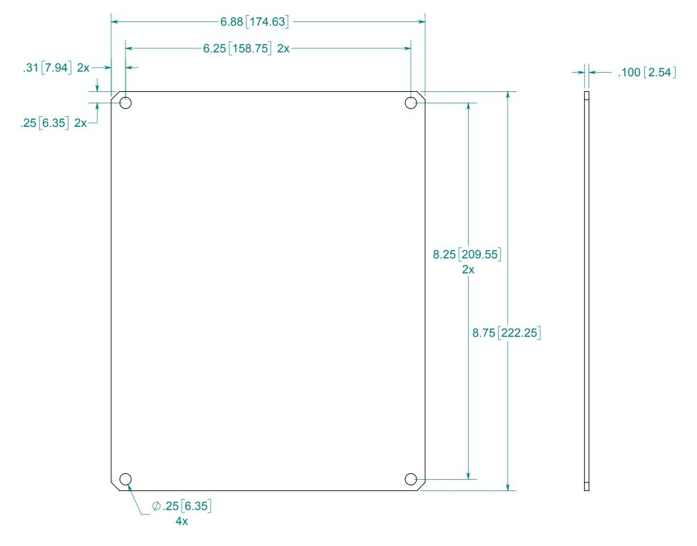
ALUMINUM 3003-H14 WITH PROTECTIVE PEEL-OFF FILM ON ONE SIDE.
