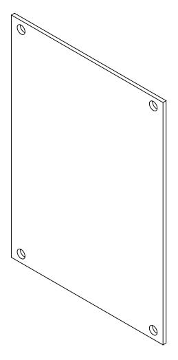
Aluminum 3003-H14 With Protective Peel-Off Film
