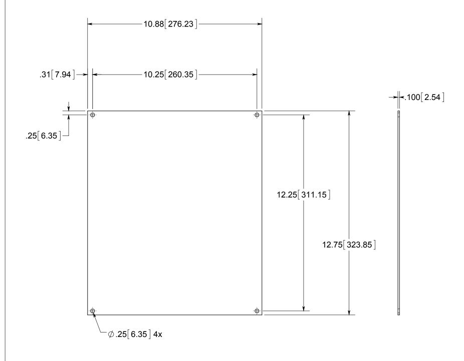
Aluminum 3003-H14 With Protective Peel-Off Film
