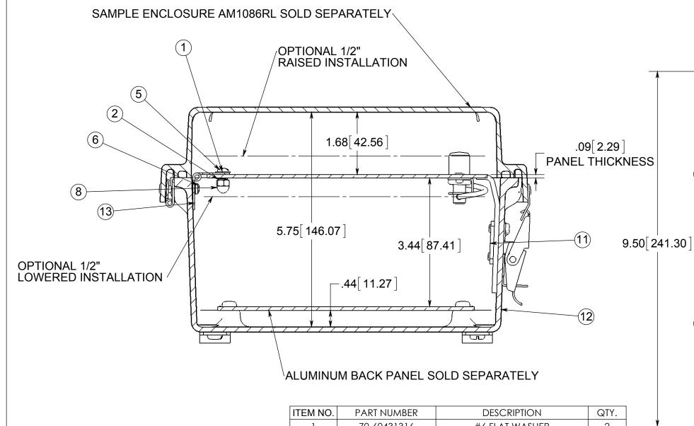
NOT ALL PARTS OF HFP ASSEMBLY KIT ARE SHOWN, ONLY THE PARTS USED IN THE FLUSH INSTALLATION OF THE PANEL. FOLLOW INSTALLATION INSTRUCTIONS INCLUDED IN THE KIT FOR THE OPTIONAL PANEL MOUNTING.
