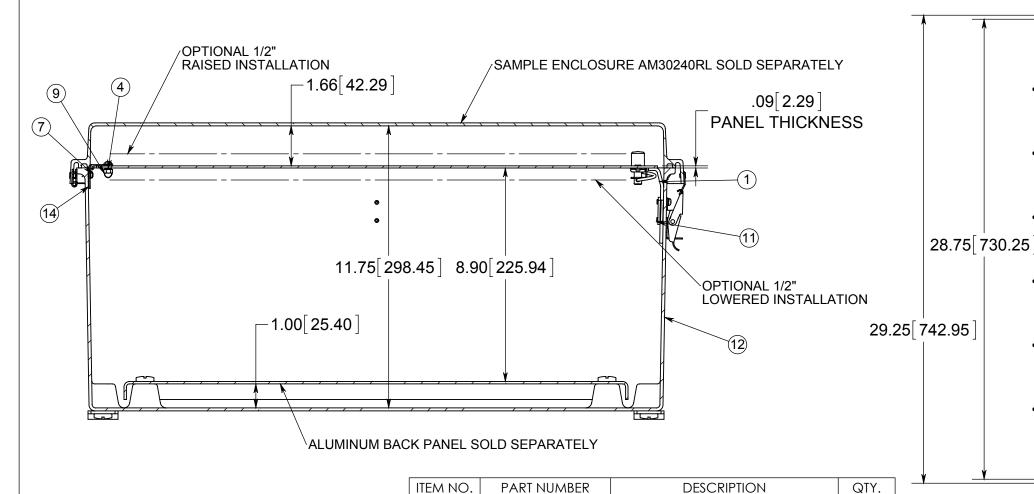
NOT ALL PARTS OF THE HFP ASSEMBLY KIT ARE SHOWN, ONLY THE PARTS USED IN THE FLUSH INSTALLATION OF THE PANEL. FOLLOW INSTALLATION INSTRUCTIONS INCLUDED IN THE KIT FOR THE OPTIONAL PANEL MOUNTING.
