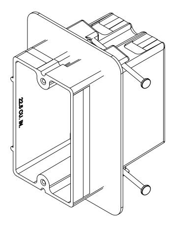
NOTES: 1.) BOX MATERIAL: FIBERGLASS REINFORCED POLYESTER, NAIL MATERIAL: PLATED CARBON STEEL, FLANGE MATERIAL: POLYURETHANE 2.) UL LISTED WITH 2 HOUR FIRE RATING FOR WALL AND CEILING
