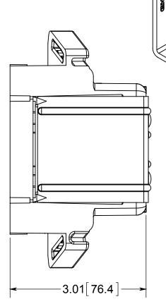
NOTES: 1.) BOX MATERIAL: FIBERGLASS REINFORCED POLYESTER, BRACKET MATERIAL: GALVANIZED STEEL, SPEED KLAMP MATERIAL: PVC
