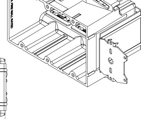
NOTES: 1.) BOX MATERIAL: FIBERGLASS REINFORCED POLYESTER, BRACKET MATERIAL: GALVANIZED STEEL, SPEED KLAMP MATERIAL: PVC
