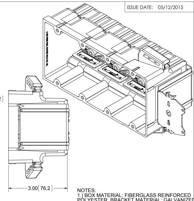
1.) BOX MATERIAL: FIBERGLASS REINFORCED POLYESTER, BRACKET MATERIAL: GALVANIZED STEEL, SPEED KLAMP MATERIAL: PVC 2.) UL LISTED WITH 2 HOUR FIRE RATING FOR
