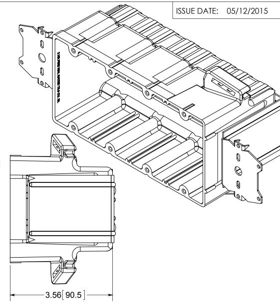
1.) BOX MATERIAL: FIBERGLASS REINFORCED POLYESTER, BRACKET MATERIAL: GALVANIZED
