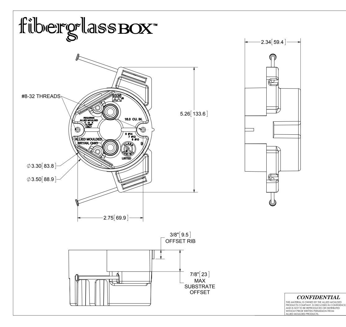
NOTES: 1.) BOX MATERIAL: FIBERGLASS REINFORCED POLYESTER, NAIL MATERIAL: PLATED CARBON STEEL, SPEED KLAMP MATERIAL: PVC 2.) UL LISTED WITH 2 HOUR FIRE RATING FOR WALL AND CEILING 3.) ANGLED MID-NAILED 4.) 2 SPEED KLAMPS FACTORY INSTALLED
