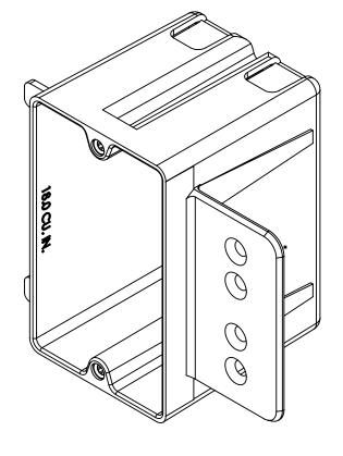
NOTES: 1.) BOX MATERIAL: PVC 2.) UL LISTED WITH 2 HOUR FIRE RATING FOR WALL AND CEILING
