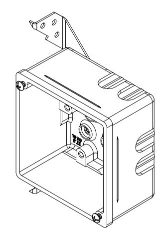
NOTES: 1.) BOX MATERIAL: FIBERGLASS REINFORCED POLYESTER, WIRE CLAMP MATERIAL: GALVANIZED STEEL, WIRE CLAMP SCREW MATERIAL: ZINC PLATED STEEL, MOUNTING BRACKET MATERIAL: GALVANIZED STEEL, MOUNTING BRACKET RIVET MATERIAL: ZINC PLATED STEEL, SCREW MATERIAL: ZINC PLATED STEEL
