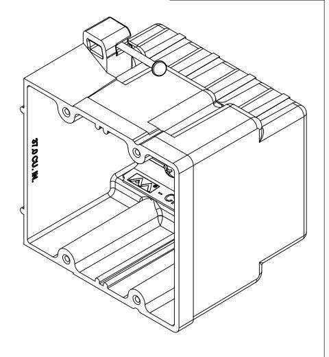
NOTES: 1.) BOX MATERIAL: FIBERGLASS REINFORCED POLYESTER, NAIL MATERIAL: PLATED CARBON STEEL, WIRE CLAMP MATERIAL: GALVANIZED STEEL, WIRE CLAMP SCREW MATERIAL: ZINC PLATED STEEL
