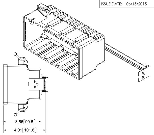
1.) BOX MATERIAL: FIBERGLASS REINFORCED POLYESTER, NAIL MATERIAL: PLATED CARBON STEEL, BAR MATERIAL: GALVANIZED STEEL, BAR MOUNTING BRACKET MATERIAL: GALVANIZED STEEL, MOUNTING BRACKET SCREW MATERIAL: ZINC PLATED STEEL, SPEED KLAMP MATERIAL: **PVC**
