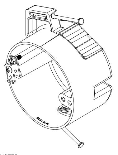
NOTES: 1.) BOX MATERIAL: FIBERGLASS REINFORCED POLYESTER, NAIL MATERIAL: PLATED CARBON STEEL, GROUND STRAP MATERIAL: GALVANIZED STEEL, GROUND MOUNTING SCREW MATERIAL: ZINC PLATED STEEL, GROUND SCREW MATERIAL: GREEN ZINC PLATED STEEL, WIRE CLAMP MATERIAL: GALVANIZED STEEL, WIRE CLAMP SCREW MATERIAL: ZINC PLATED STEEL 2.) UL LISTED WITH 2 HOUR FIRE RATING FOR WALL AND CEILING
