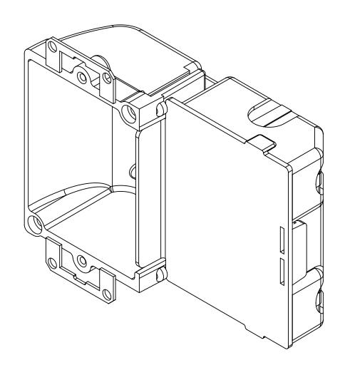
.52[13.13] OFFSET 1.69 42.88 1.17 29.74 NOTES: 1.) BOX MATERIAL: FIBERGLASS REINFORCED POLYESTER, EAR MATERIAL: GALVANIZED STEEL 2.) UL LISTED WITH 2 HOUR FIRE RATING FOR WALL AND CEILING
