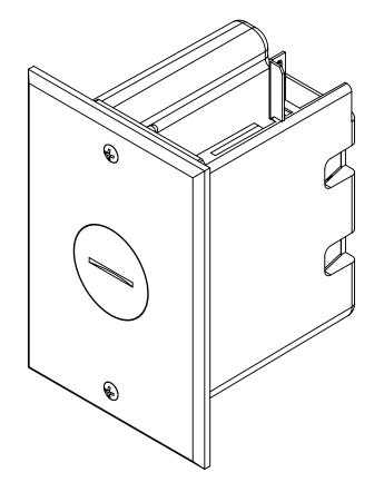
NOTES: 1.) BOX MATERIAL: POLYCARBONATE, COVER PLATE MATERIAL: NICKLE PLATED BRASS, COVER PLATE MOUNTING SCREW MATERIALS: NICKLE PLATED BRASS, DEVICE MOUNTING SCREW MATERIALS: ZINC PLATED STEEL, FLANGE MOUNTING SCREW MATERIALS: BLACK PHOSPHATE COATED STEEL WING MATERIAL: ZINC PLATED STEEL, GROUND PLATE MATERIAL: ZINC PLATED STEEL, GASKET MATERIALS: POLYURETHANE FOAM 2.) UL LISTED, FLOOR BOX MEETS UL514C SCRUB WATER EXCLUSION TEST
