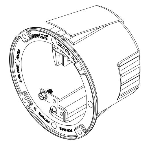
1.) BOX MATERIAL: FIBERGLASS REINFORCED POLYESTER, SNAP BRACKET MATERIAL: GALVANIZED STEEL, SNAP BRACKET SCREW MATERIAL: ZINC PLATED STEEL, GROUND STRAP MATERIAL: GALVANIZED STEEL, GROUND STRAP MOUNTING SCREW: ZINC PLATED STEEL, GROUND SCREW MATERIAL: GREEN ZINC PLATED STEEL, SPEED KLAMP MATERIAL: PVC 2.) UL LISTED WITH 2 HOUR FIRE RATING FOR WALL AND CEILING 3.) 2 SPEED KLAMPS FACTORY INSTALLED
